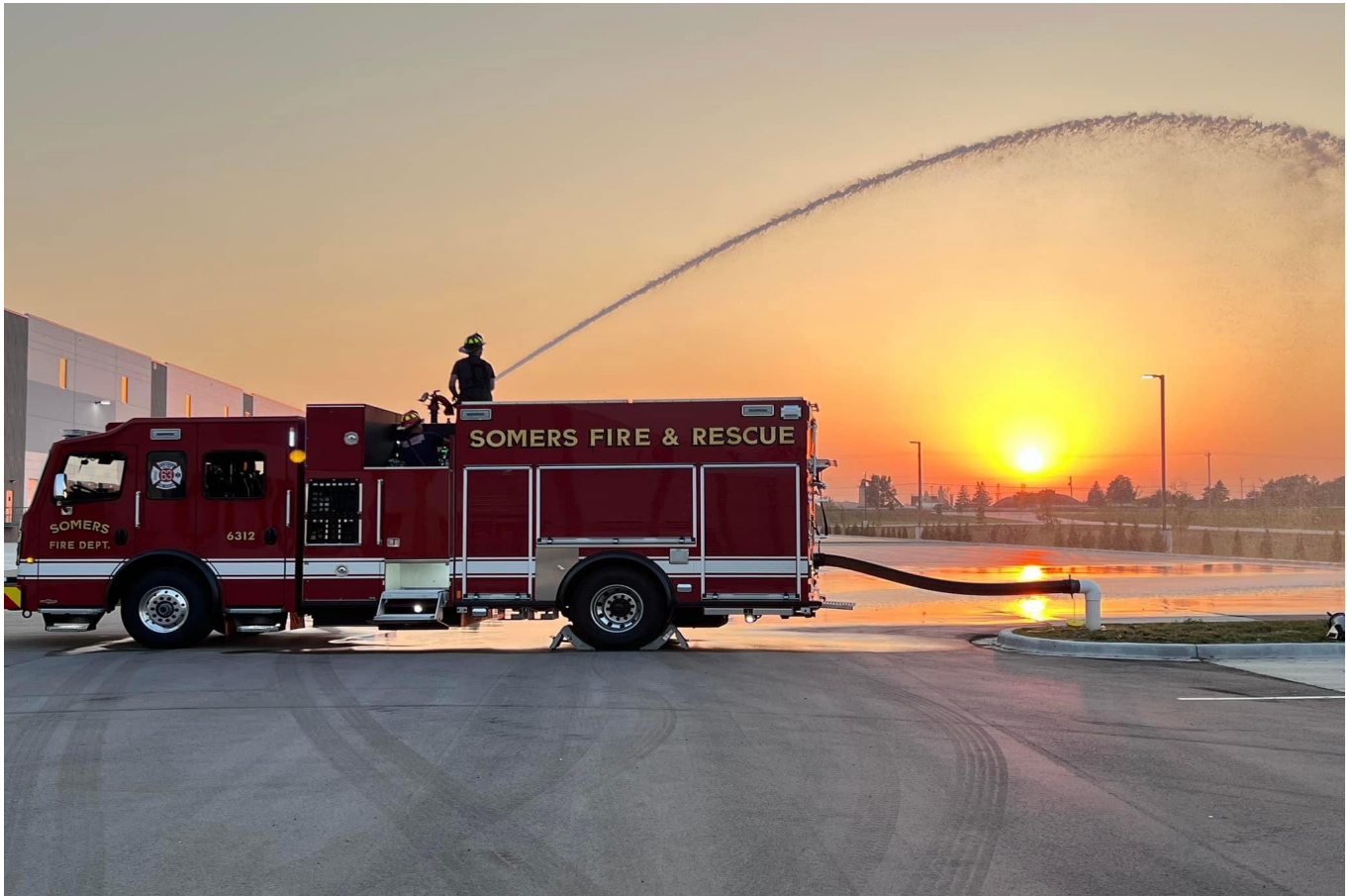
Somers Fire Department pump operators practice drafting (sucking water) from ponds at local warehouses.
